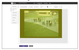
**4.** On the **Calibration** tab, set the location and orientation of the camera.
